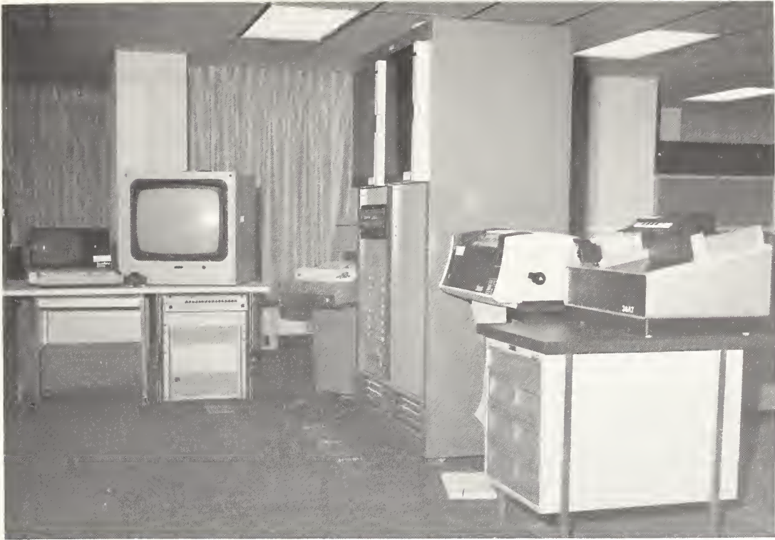
Figure 11-3.--MMIPS configuration (l to r): Keyboard/alphanumeric CRT; color imager CRT; teletypewriter; GTE minicomputer, tape units, line printer, and card reader. Not shown--two 22-M byte Ampex disk units.
